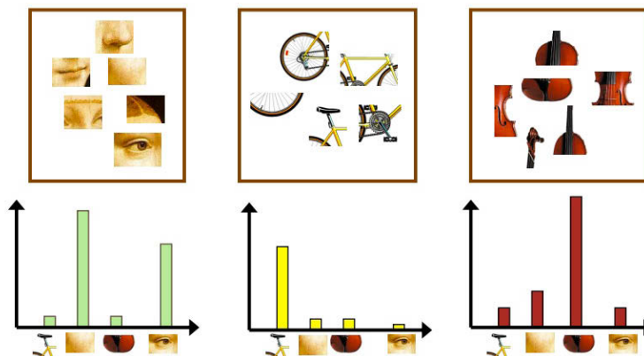
Figure 5: Using a bag-of-words model, image feature vectors are expressed by a histogram of the occurrences of representative descriptors within the image. Different levels of descriptor occurrence can provide information about the contents of an image.
