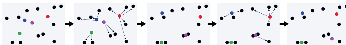
Figure 4: K-means clustering is an algorithm used to group data points into k clusters based on similarity. Centroids are represented as colored circles and data points are represented as dark circles.
